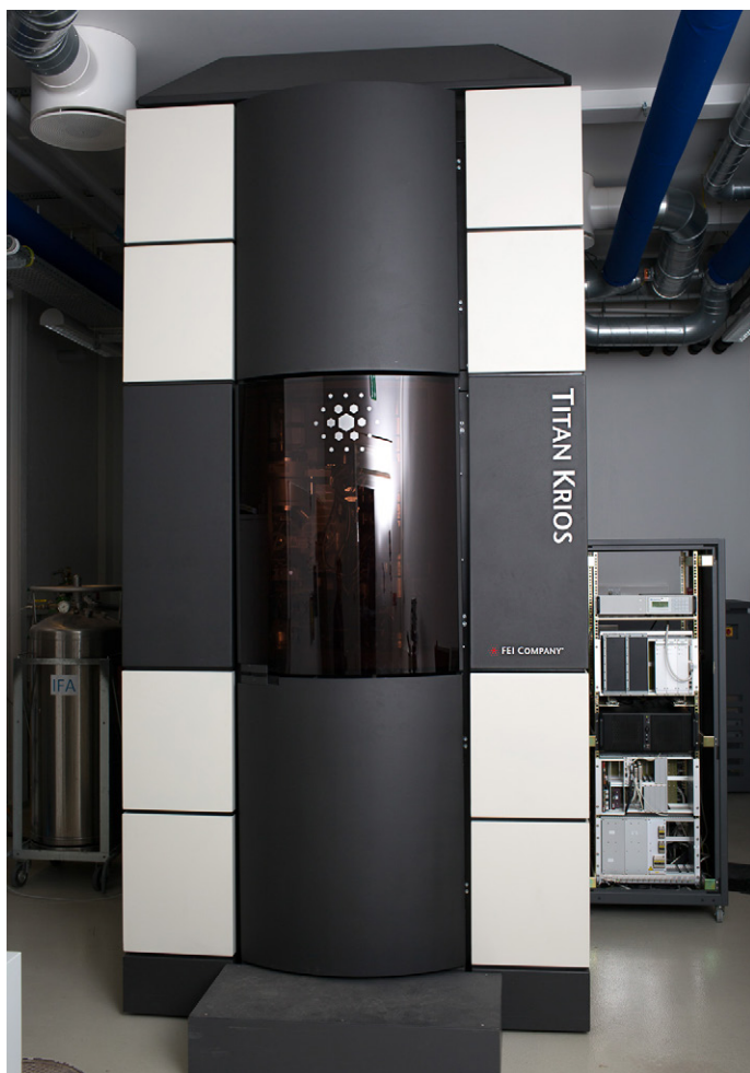
Fig. 1. The TITAN Krios TEM available at AU provides a state-of-the art facility and can be used to obtain high-resolution images from macromolecular machines. Data collection is fully automated and images are processed in a highly streamlined manner on a powerful computer cluster. Photo by Lars Kruse, AU Komm.
