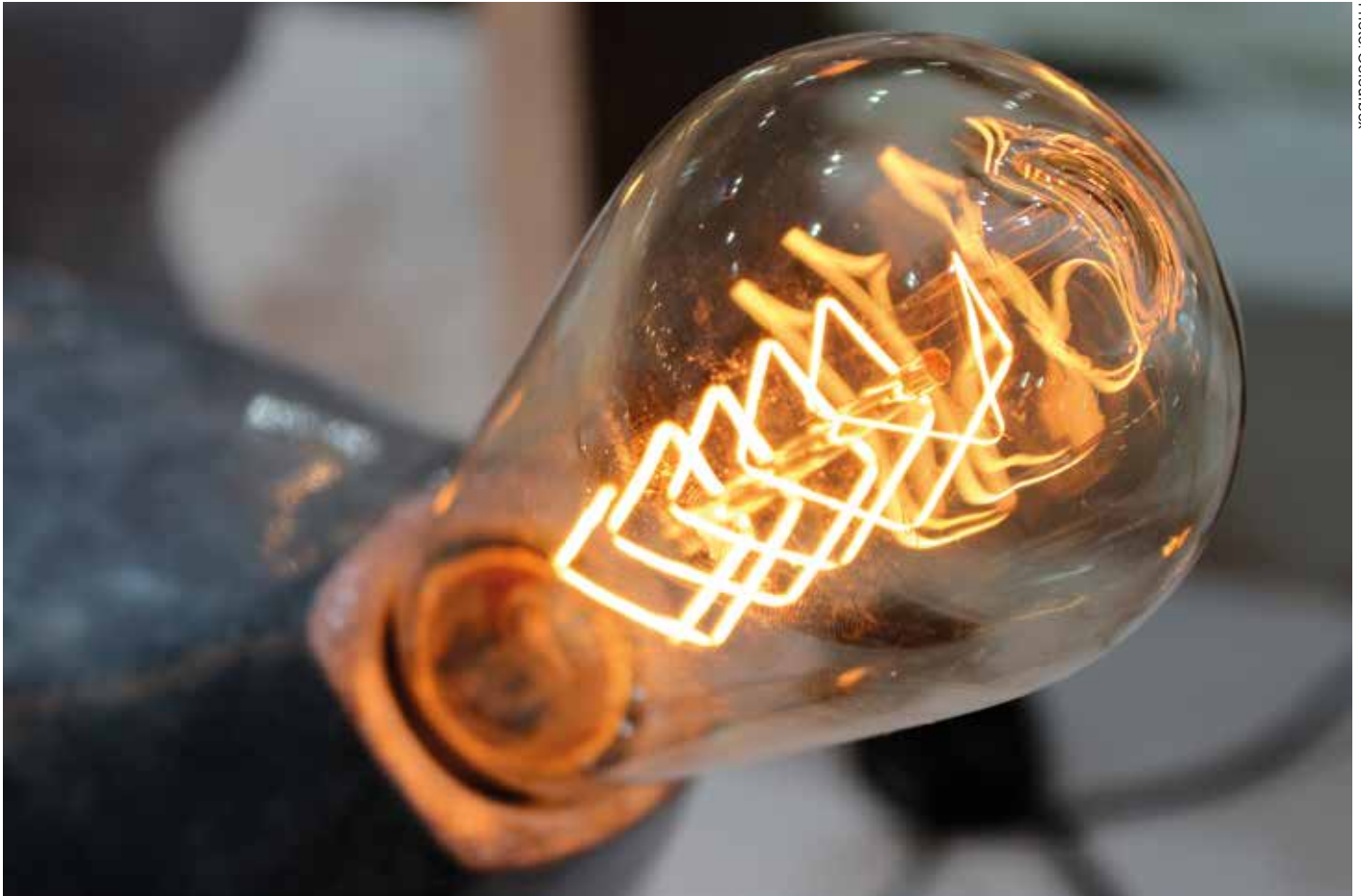
Incandescence – the heating of a wire filament with electricity to such a high temperature that it glows with visible light. The invention, which has been attributed to Thomas Edison, sparked a revolution fundamental to our society and way of life today.
