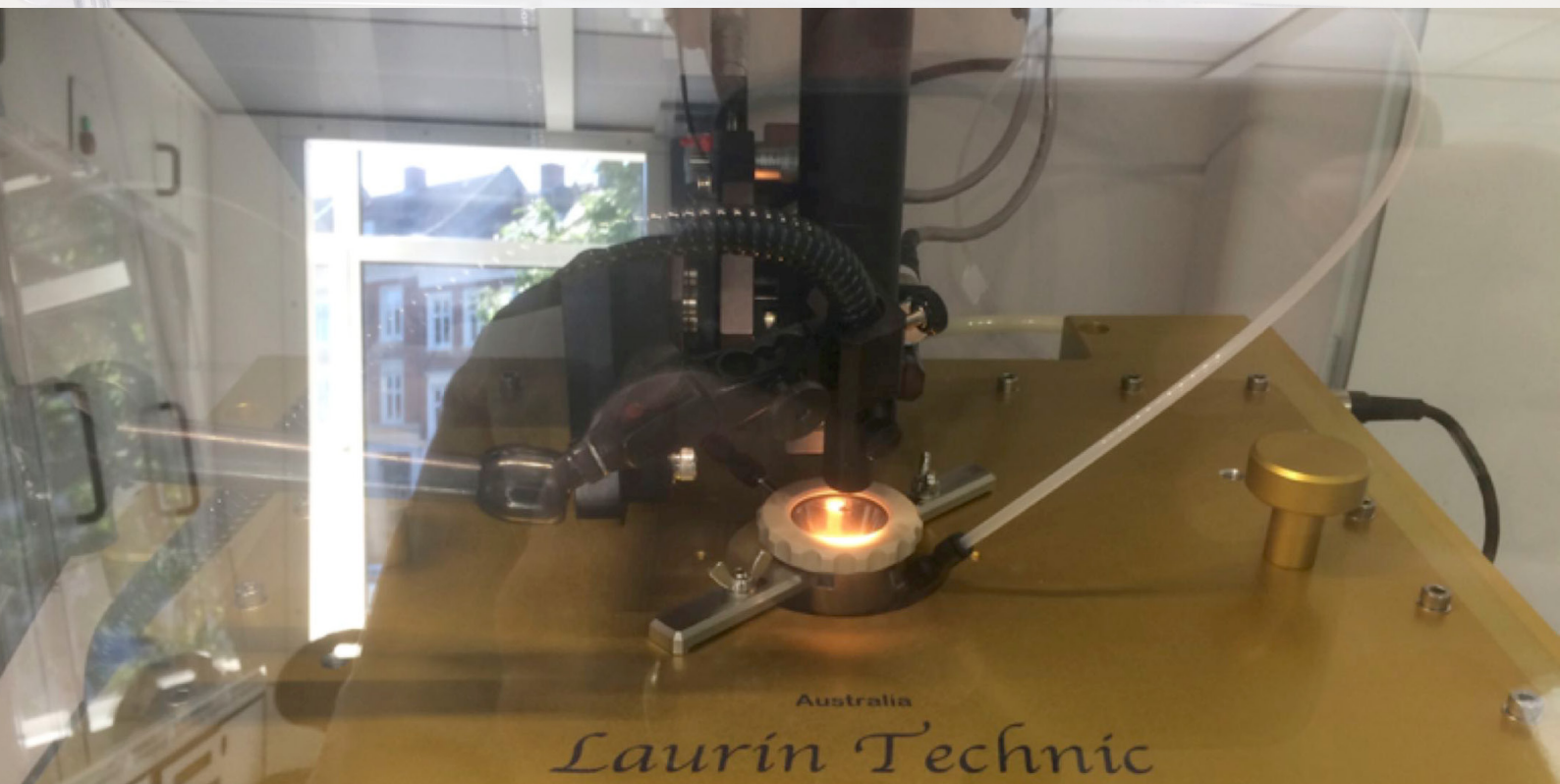
Double exposure of 193 nm (wavelength) Nd: YAG laser connected to mass spectrometer for in-situ trace-metal and isotopic analysis of artefacts (foreground) and metal-free, ultra-clean laboratory for chemical purifications of digested samples for isotopic analysis (background) (Photo: Charles Lesher).
