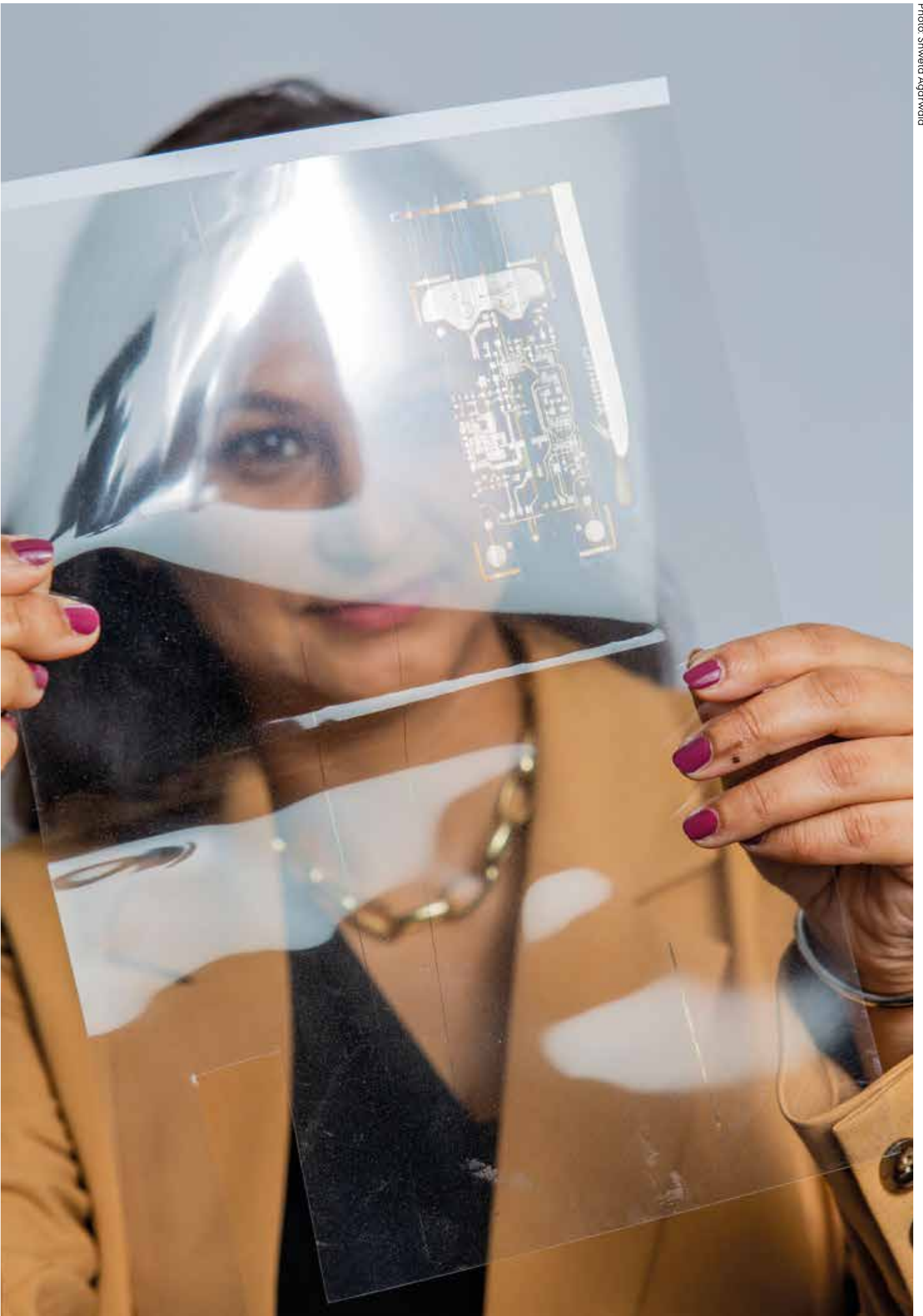
Assistant Professor Shweta Agarwala is combating e-waste with new, completely biodegradable electronics.
