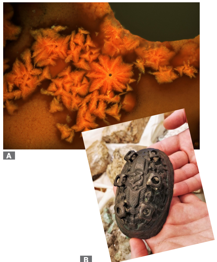
A: Copper oxides in the crucible slag (© Vana Orfanou). B: An oval brooch from the early Viking period (early 9th century CE) (© Søren M. Sindbæk).
