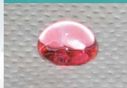
A drop of water on a superhydrophobic nonwoven.
