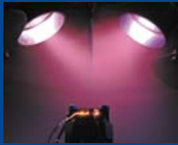
Left: Deposition with two magnetrons. Right: Schematic of magnetron sputtering.
