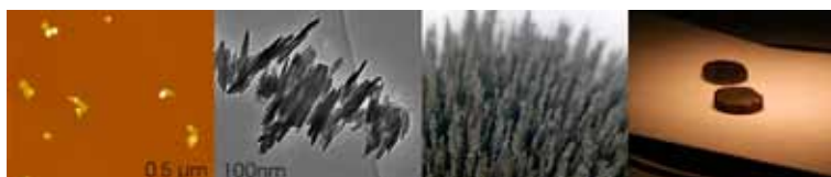
Production (left to right) of magnetic pellets: cheap metallic salts are dissolved in water and crystallized. The resulting magnetic nanoparticles are imaged by AFM microscopy and TEM microscopy. Photographs show the nanopowder and final mm-cm sized pellets.
