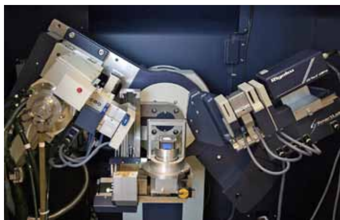
The instrument is a Rigaku X-ray diffractometer. The X-ray source is mounted on the left hand side and the sample is found in the middle, while the detector is seen to the right. The emitted X-rays are reflected by the atomic planes in the nanocrystals and the angular positions and intensities of these reflections gives information about their structures at the atomic level. A structure of a single domain magnetic nanocrystal is shown above
