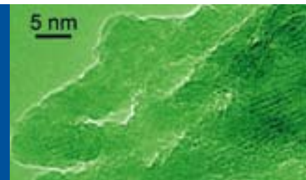
By controlling synthesis conditions, we can manipulate the size and shape of nanoparticles. The image is of apatite nanocrystals taken with the transmission electron microscope. The striations seen within the crystals reveal the underlying crystal lattice.
